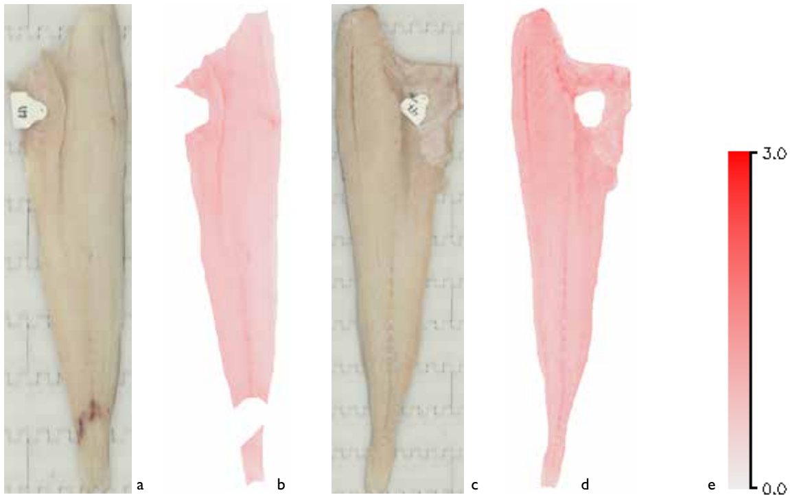
Figure 5.27: a) and c) shows color images of two cod fillets, and b) and d) shows corresponding blood response for those fillets. e) shows color coding for blood response values between 0.0 and 3.0.
