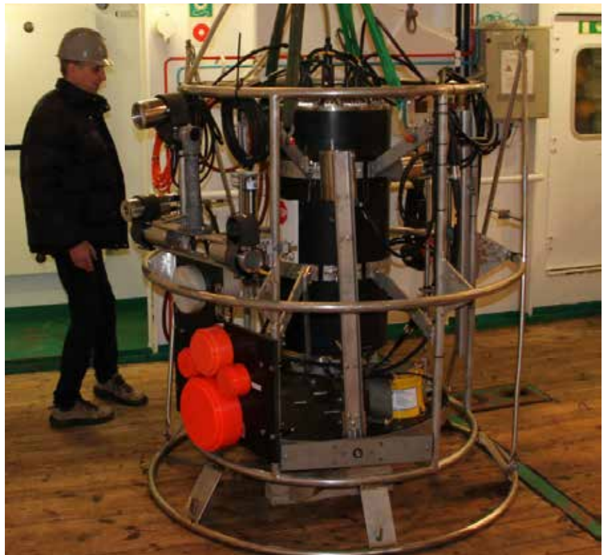
Figure 5.1: The TS probe, used to measure individual target strength of single mackerel in dorsal (echo sounder mode) and lateral (sonar mode).
