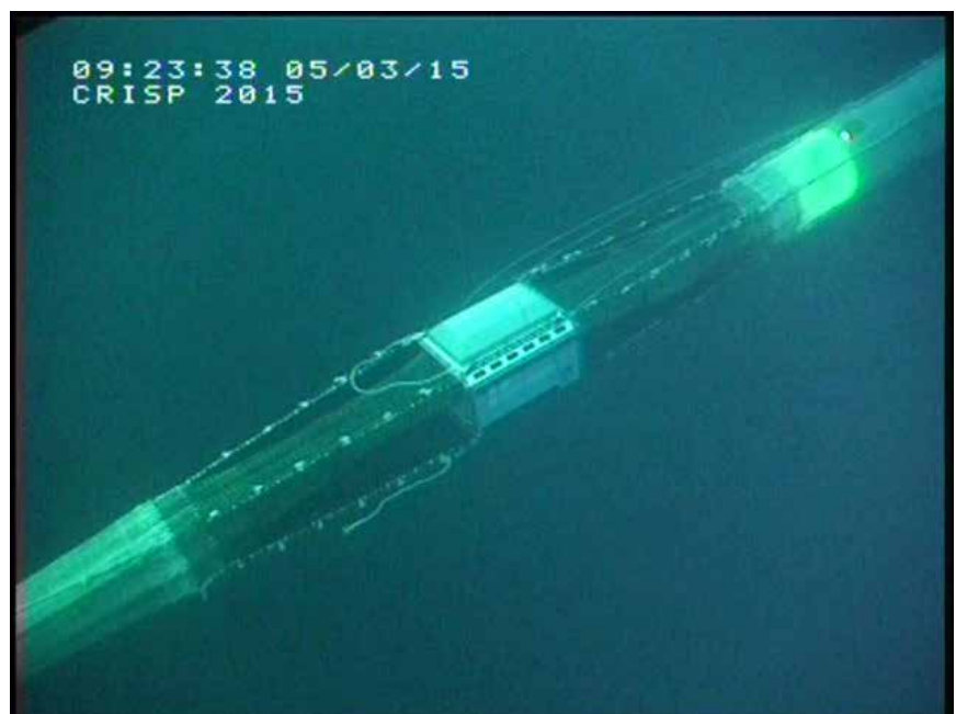
Figure 5.13: Deep Vision during deployment on CRISP cruise in March, 2015. Deep Vision frame at centre, 3 m long leading sections are the dark mesh panels before (right) and after (left) the Deep Vision frame.
