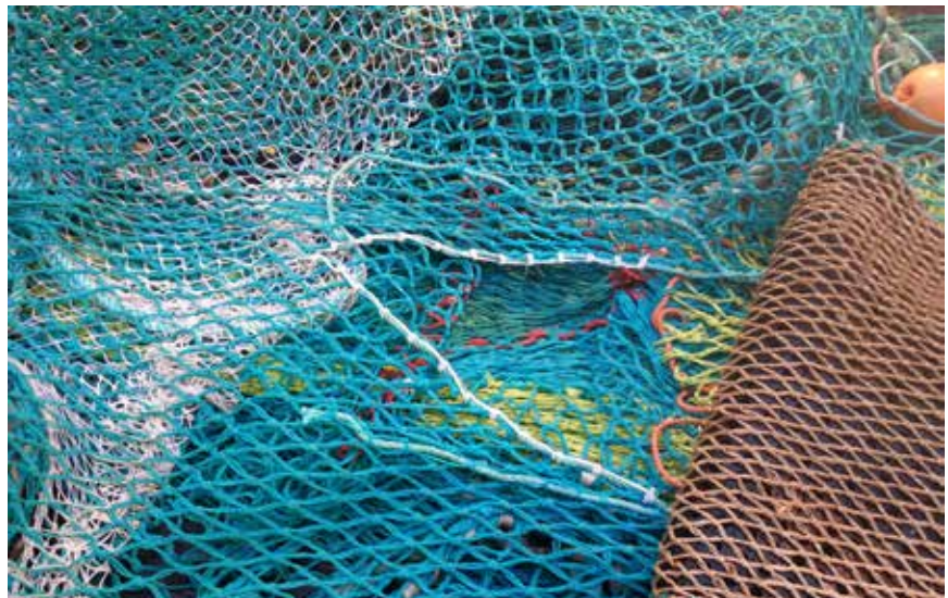
Figure 5.22: The original square release opening in exfed was replaced by a triangular one pointing backwards. the brown cover mat to the right.
