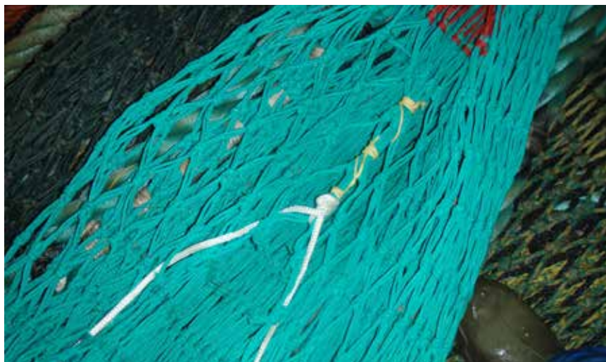
Figure 5.23: The demersal seine system: a slot cut in the upper panel, kept closed during towing with a rope or a thick twine.
