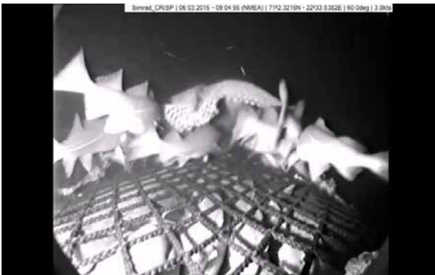
Figure 5.17: The live Simrad FX80 trawl camera was used to document the escape of fish through the catch limitation device (CRISPWVP4).
