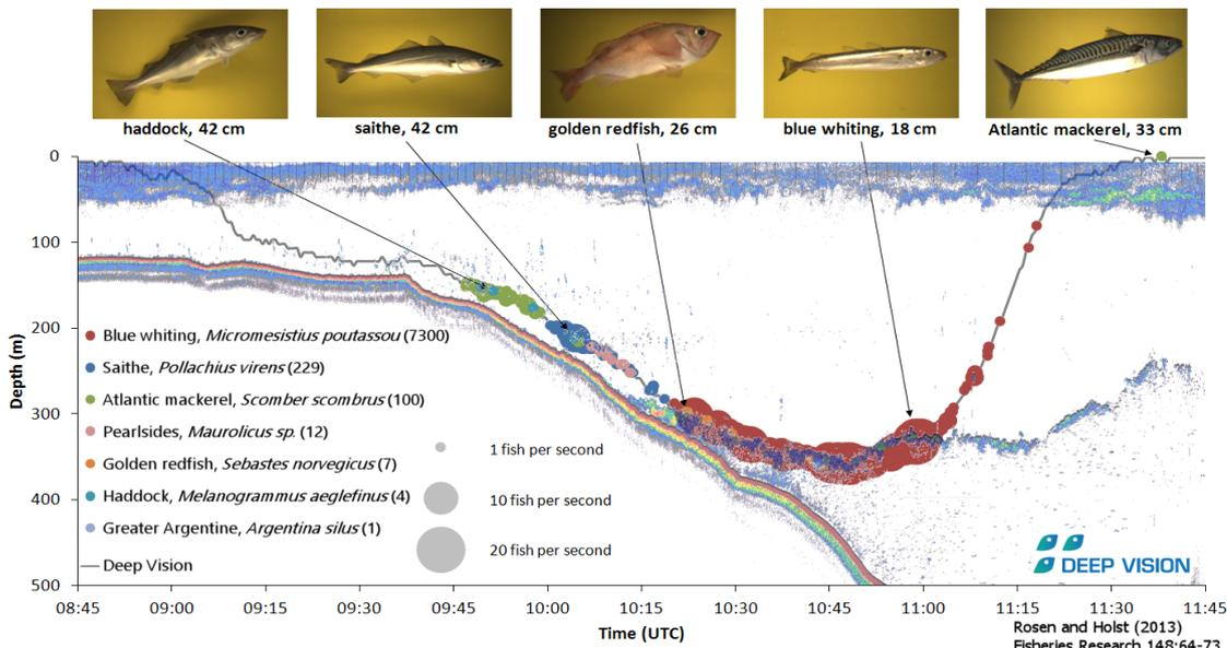
DEEP VISION OVERLAYED WITH SONAR DATA: Deep Vision is an invaluable tool in acoustic mapping of resources. All images are logged with information about time and depth. Combined with sonar data the system shows the density of different species along the haul.
