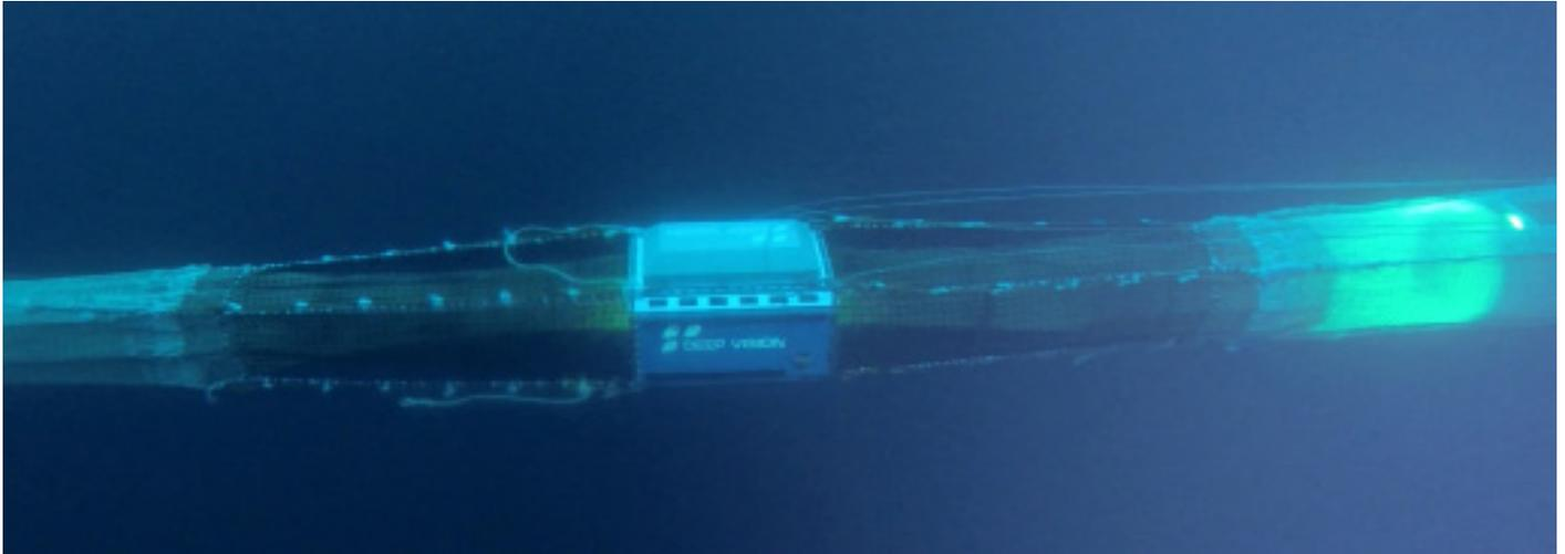
**DEEP VISION FRAME UNDER WATER:** The Deep Vision frame is attached to the trawl and records images of all organisms passing through. This unique approach to fish sampling enables research to be done without bringing the fish onboard the vessel. PHOTO: Jan Tore Øvredal/CRISP
