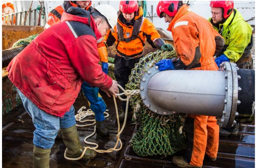
**Figure 5.1.** The crew is tightening the codend to the pump hose (Photo: © NOFIMA).
