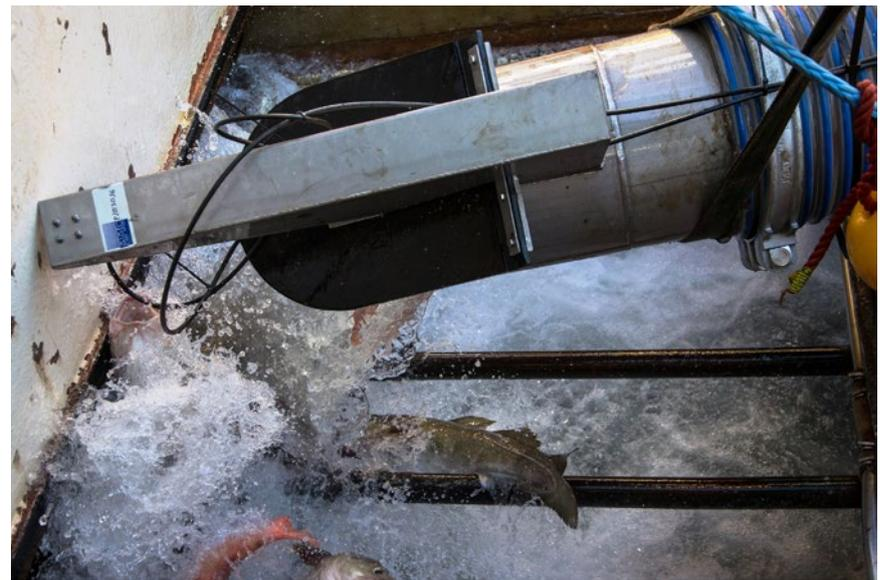
**Figure 5.2.** The vacuum pump delivered 20 tonnes per hour and the fish was pumped down into the trawler's receiving bins (Photo: © NOFIMA).
