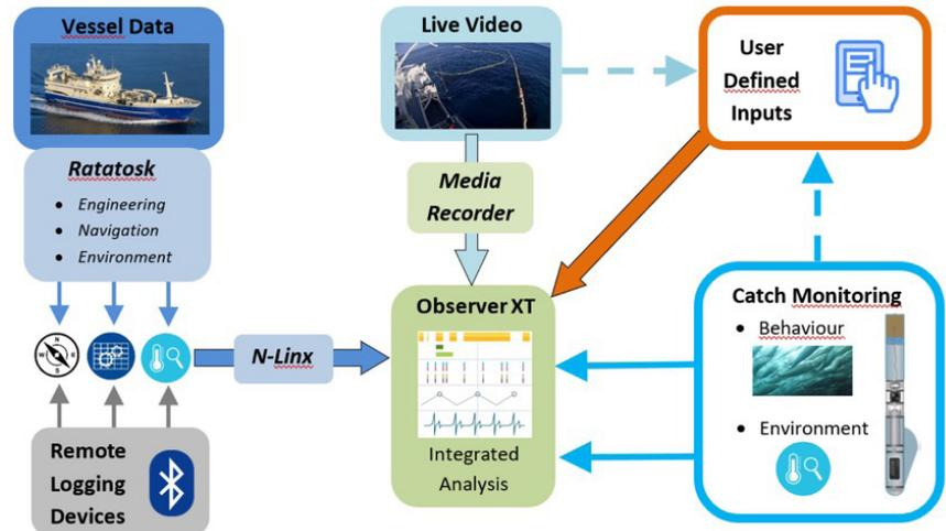
Figure 5.2.5. An overview of the compilation and integration of data (behavioural, engineering, environmental, and navigational) from several sources (vessel, live video, remote logging devices, catch monitoring devices and user defined inputs) via the Ratatosk, N-Linx, Media Recorder and Observer XT systems (Source: Catch Control in Purse Seine - <https://www.sintef.no/projectweb/ffangstkontroll/>).
