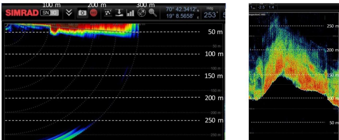
Figure 5.2.1. Vertical section of a capelin school using SN90 sonar with the closer edge of the school at 100 m at a depth of 20 m (left panel). An inspection beam oriented perpendicular to the school, show the decrease (from red to light green colour) in the acoustic backscattering from the closer part of the school at about 100 m towards the distant border about 170 m from the vessel. The range indicates, horizontal distance from the vessel (right panel).
