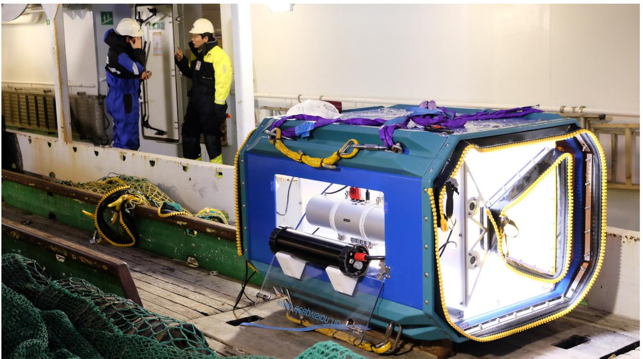
Figure 5.3.1. Deep Vision electronics and new deployment frame. Photo Tim Petter Hansen, UiB.
