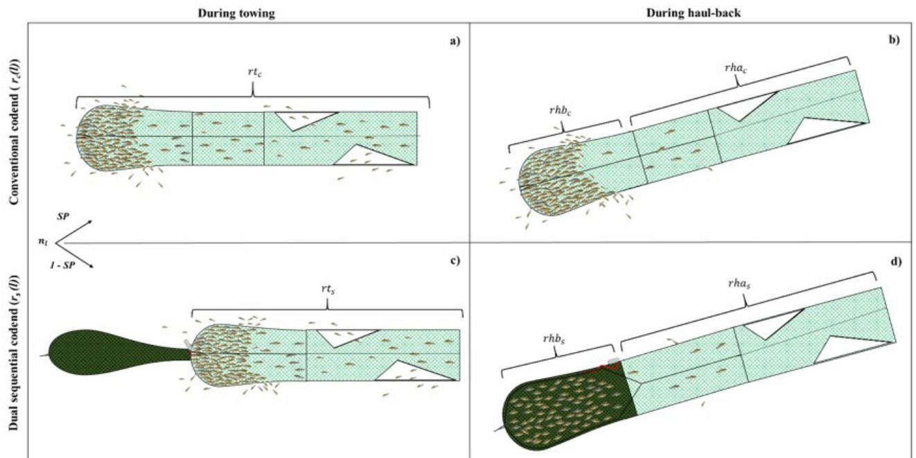
Figure 5.5.2. Schematics showing the size selectivity that occurs with the conventional codend ( $rc(l)$ ) during (a) towing and (b) haul-back. (c) Size selection in the anterior codend segment of the dual sequential codend during towing, which, due to the codend design, (d) should cease during haul-back when the fish enter the posterior quality-improving codend segment. (The sections are not scaled according to each other).
