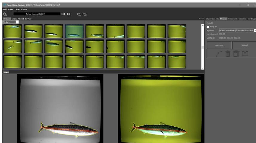
Figure 5.3.2. Example of automatic segmentation, object matching in left and right images, and calculation of length. In this example, the midline of the selected Atlantic mackerel (*Scomber scombrus*) is generated as a series of 25 segments, with a total length of 350 mm. Image courtesy Girona Vision Research SL.
