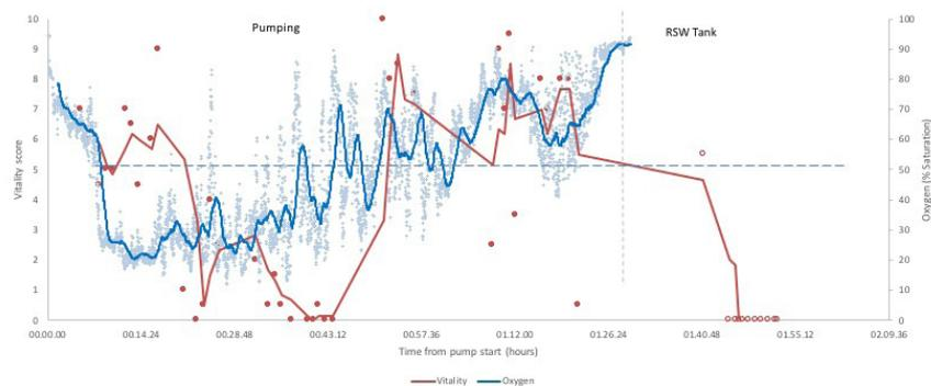
Figure 5.2.4. oxygen concentrations can become very low in the catch during pumping because of high crowding densities, which can significantly affect the “vitality” of the fish as they are pumped on board.
