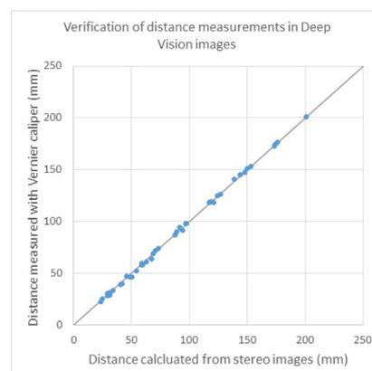
Figure 5.3.4. Distances measured from Deep Vision images ( $x$ -axis) match well with physical measurements made using Vernier caliper. Grey line is expected 1:1 relationship. Fifty-one percent of values were accurate within 1 mm, maximum error was an underestimate by 4.5 mm over a 50 mm interval.
