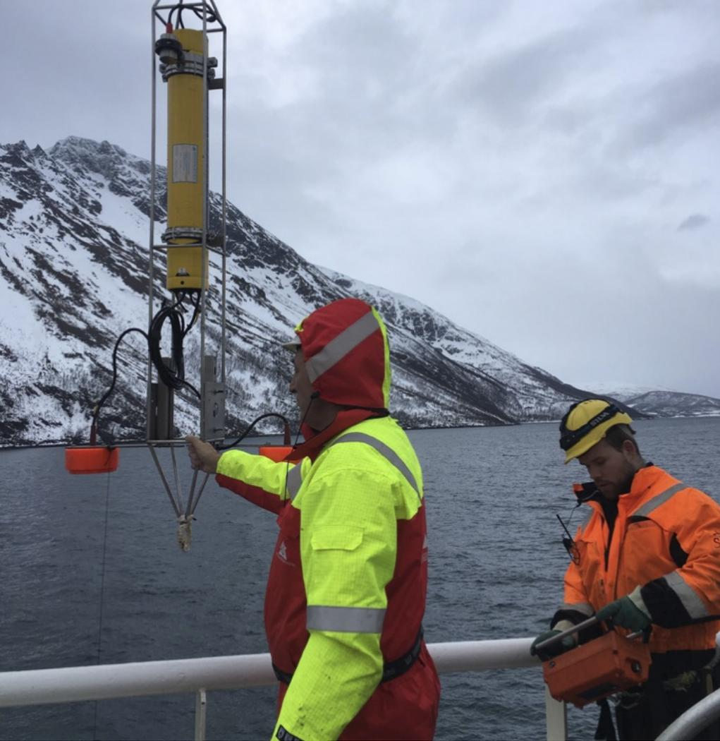
Figure 5.1.4. Setting out the WBAT system for target strength measurements.
