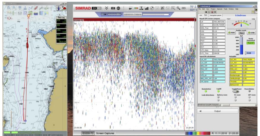
Figure 5.1.2. KayakDrone used on herring layers in Kvanøngen, showing the echogram recorded onboard the Drone while passed by RV “G.O.Sars”. The herring reaction to the research vessel was obvious as they started diving 100 meters in front of the vessel. Comparisons between densities measured from the vessel, from a drifting buoy, from the Drone and from the side-looking MS70 system will be made on this dataset.
