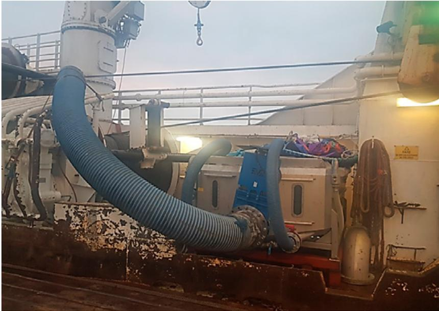
Figure 5.5.4. The new live storage tank installed at the trawl deck onboard FV “J. Bergvoll”, Nergård Havfiske AS (Photo: Nofima AS).
