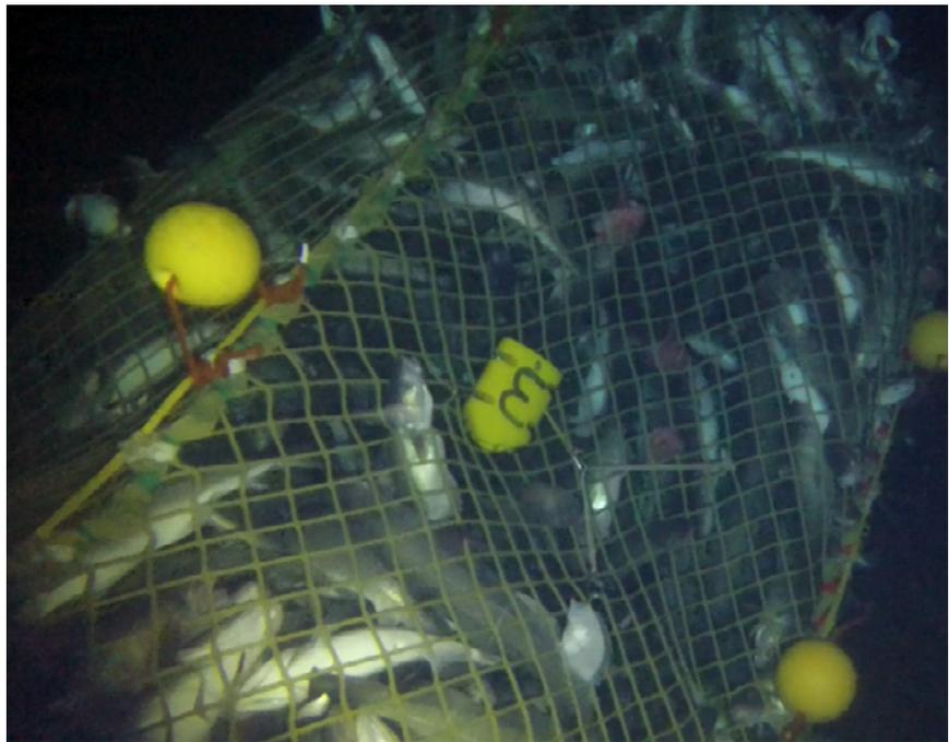
*Figure 5.4.3: Snapshot from underwater video, showing the four panel codend during towing.*
