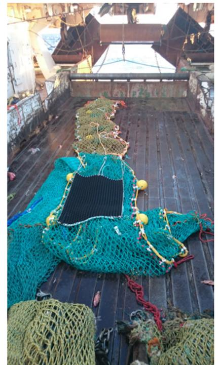
Figure 5.4.1. The four panel codend with the ExFed system. The picture is taken onboard the trawler “J. Bergvoll”.
