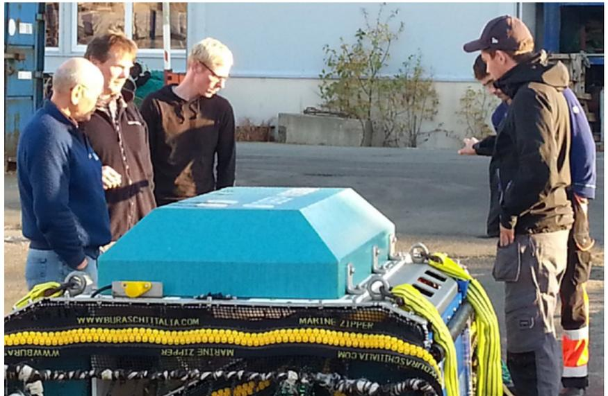
Figure 5.3.3. Kristoffer Lovall of Scantrøl Deep Vision AS explains the Deep Vision system to the crew of Nergård Havfiske's trawler "Kasfjord" which was docked at the same pier. The yellow SIMRAD transducer used for acoustic transfer is visible in front of the blue floatation block. The yellow zippers were also tested to provide ready access to clean and adjust components inside the frame.
