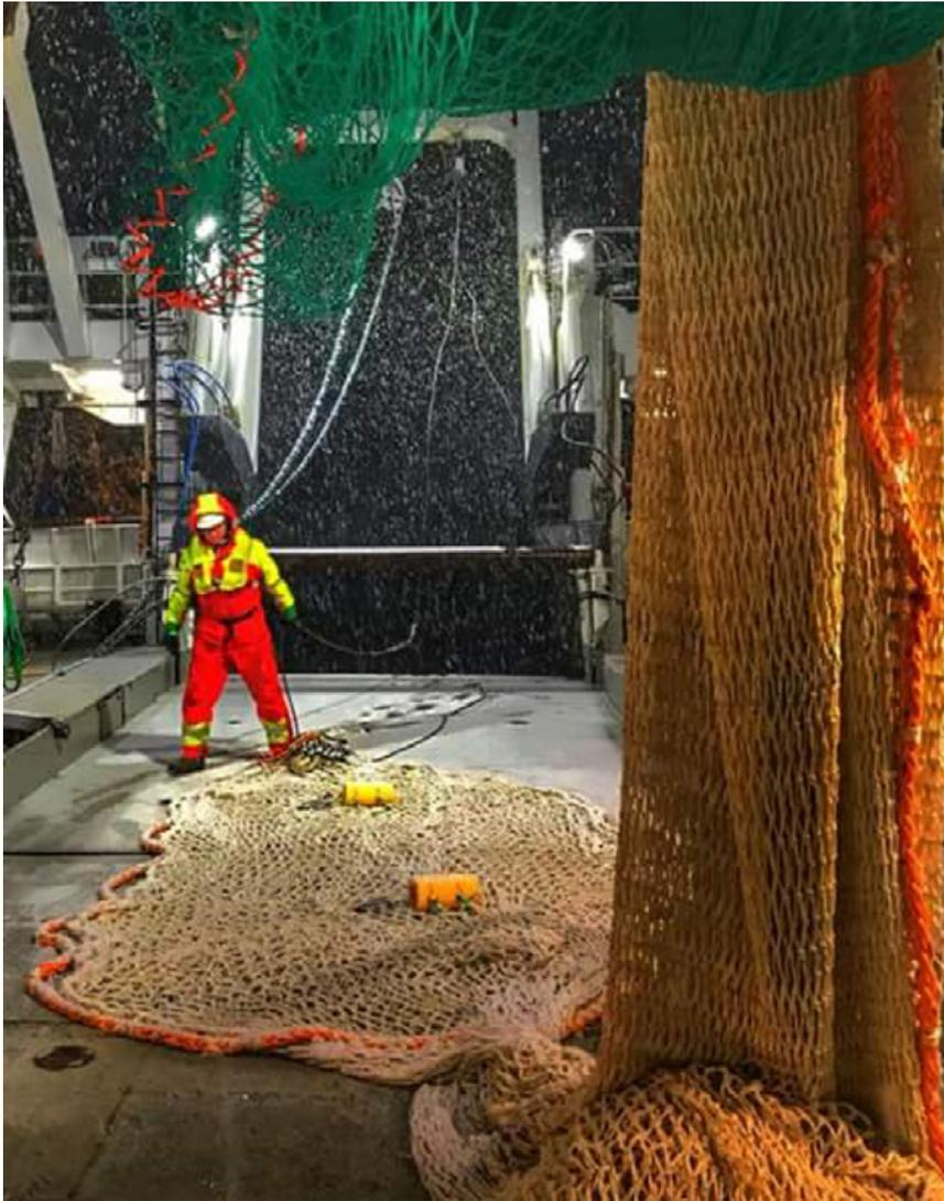
Figure 5.4.4. Fitting sensors to the trawl at the RV “Johan Hjort”-survey in December 2017 (Photo Thor Børhaugen).
