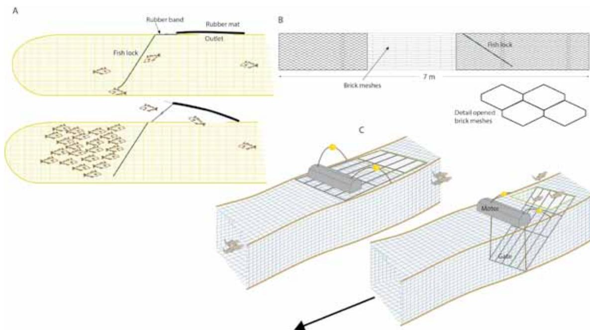
**Figure 5.6.** The three systems developed to release fish at depth. System A and system B are passive using a rubber mat covering a steel framed escape opening and brick meshes to create an escape opening, while system C is an active system using an acoustically activated motor to control a gate that blocks the codend and open the escape opening.
