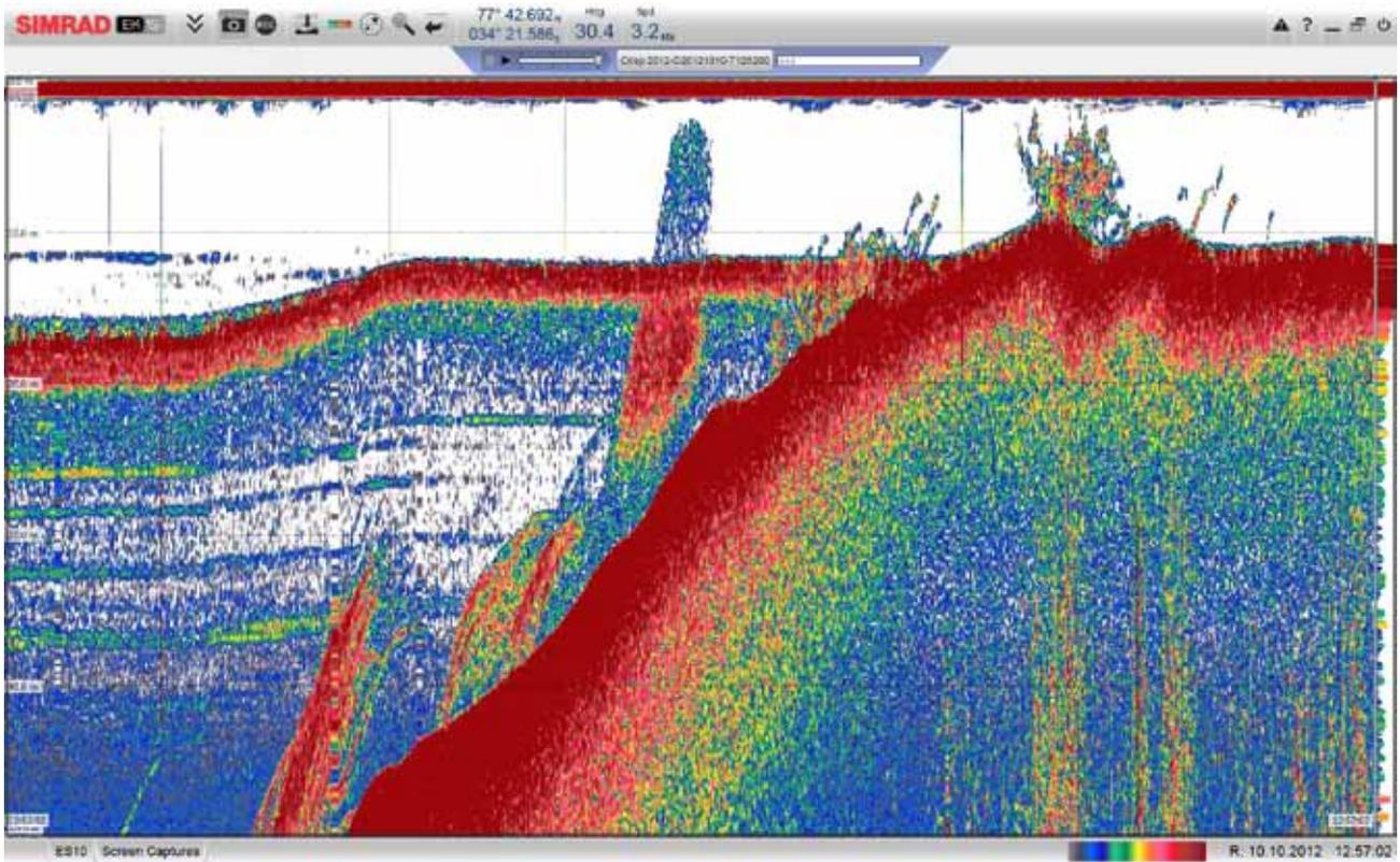
**Figure 5.4. Echosounder image showing the trawl settling on the seabed. Fish can be observed above and below the groundgear.**
