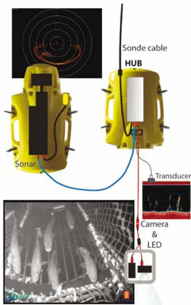
Figure 5.3. A system for observing fish and trawl behaviour by sonar, camera and echosounders.
