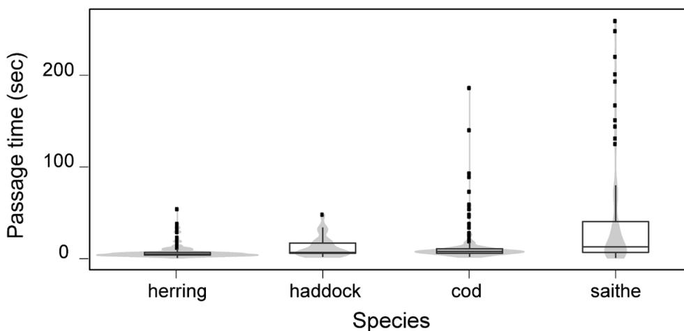
Figure 5.13. With the addition of the 8-m long tapered section, most saithe and other fish species passed through the Deep Vision with less than a minute's delay (data from February 2016 CRISP cruise).
