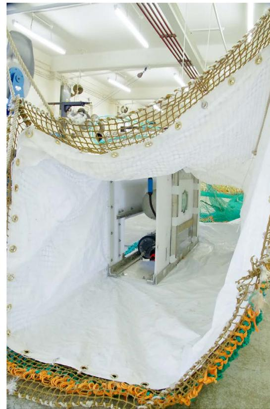
Figure 7.1. Testing of a down-scaled version of Deep Vision onboard the research vessel “Alba na Mara” in November, 2016 in the Moray Firth, west of Fraserburgh, Scotland. In this version the camera system is mounted inside a canvas cover instead of a solid frame.
