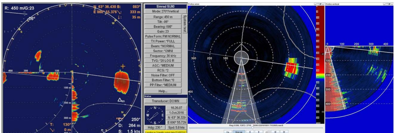
Figure 5.1. A mackerel school used in the verification work, where the school first was encircled by the vessel (FV “Brennholm”) and measured, and subsequently fished. The catch was 203 tonnes. Left panel: sonar display, Right panel: raw data during processing in PROFUS.
