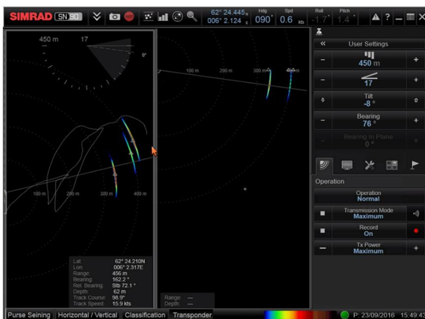
The current sonar software version allows either a Transponder Mode or a Purse Seine Mode (which is the normal view for school inspection) but not an integrated mode, where the transponders can be visualized together with the target schools in the same screen. Therefore, it was not possible to test the transponders during a purse seine shot targeting a mackerel school. Instead, an empty set was performed inside Sulafjorden to test the transponders attached to the bottom line of the purse seine.
