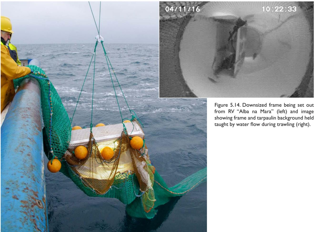
Figure 5.14. Downsized frame being set out from RV “Alba na Mara” (left) and image showing frame and tarpaulin background held taught by water flow during trawling (right).
