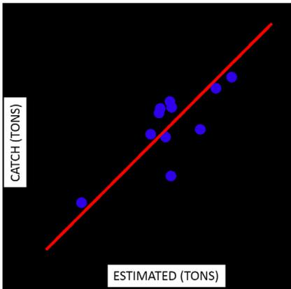
Figure 5.2. Preliminary correlation between sonar volume estimate and validation catches for Atlantic mackerel. Improvements in TS and other parameters is now made.
