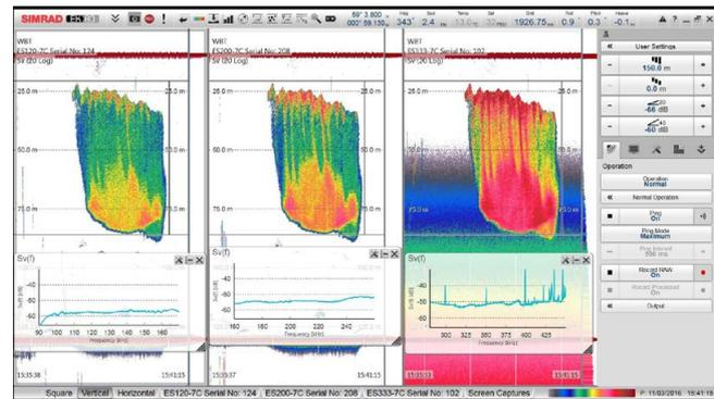
Fig. 5.3. A relatively large mackerel school, shown at three broadband frequencies, 90-160 kHz, 160-260 kHz and 260-450 kHz. SV spectrum shown below each figure.
