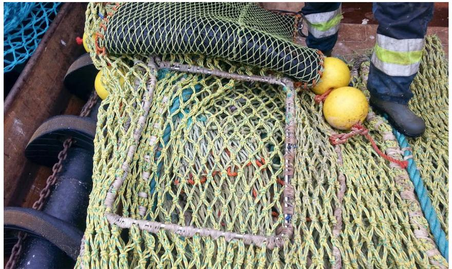
Figure 5.18. The ExFed system as previously used with a supporting steel frame to the left. To the right, the same system modified by removing the frame.
