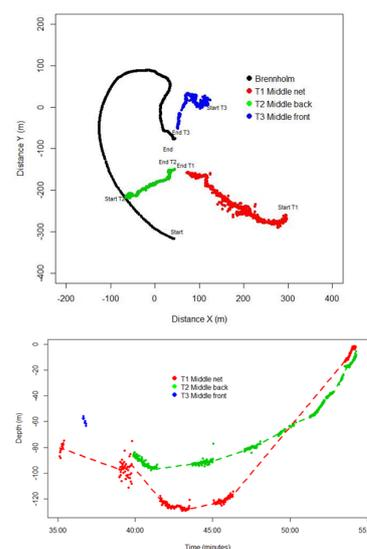
Figure 5.11. Monitoring three transponders during an empty set inside Sulafjorden. Positions in the horizontal plane of the three transponders and the vessel track (top panel). Depth of the transponders during the setting (from minute 35 to 43) and pursuing (from minute 43 to 55) of the seine (bottom panel).
