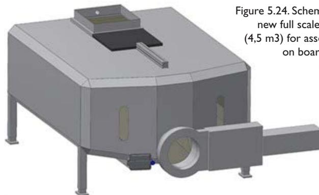
Figure 5.24. Schematic diagram of a new full scale live storage tank (4,5 m<sup>3</sup>) for assembly and testing on board FV "J. Bergvoll". (Photo: Optimar)
