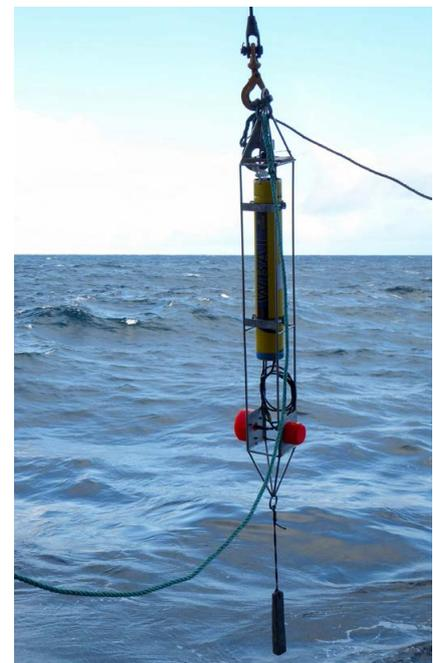
Figure 5.4. Simrad WBAT system with 70 and 200 kHz transducers, dropped into herring schools for measuring mean lateral TS of mackerel. Very good videos from inside the mackerel schools were also obtained in the 2016 survey.
