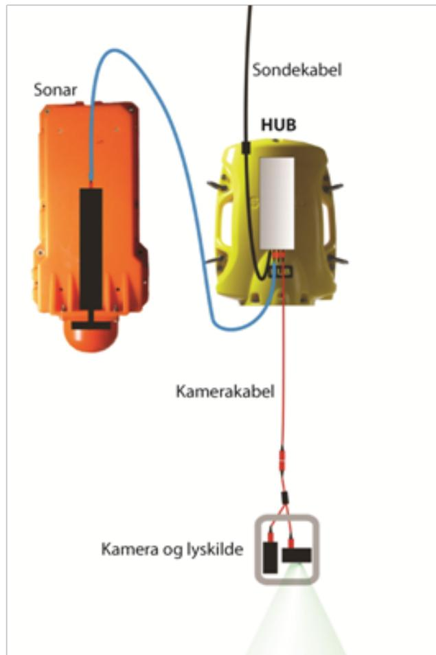
**Figure 5.2:** A system for observing fish and trawl behaviour by sonar and camera.
