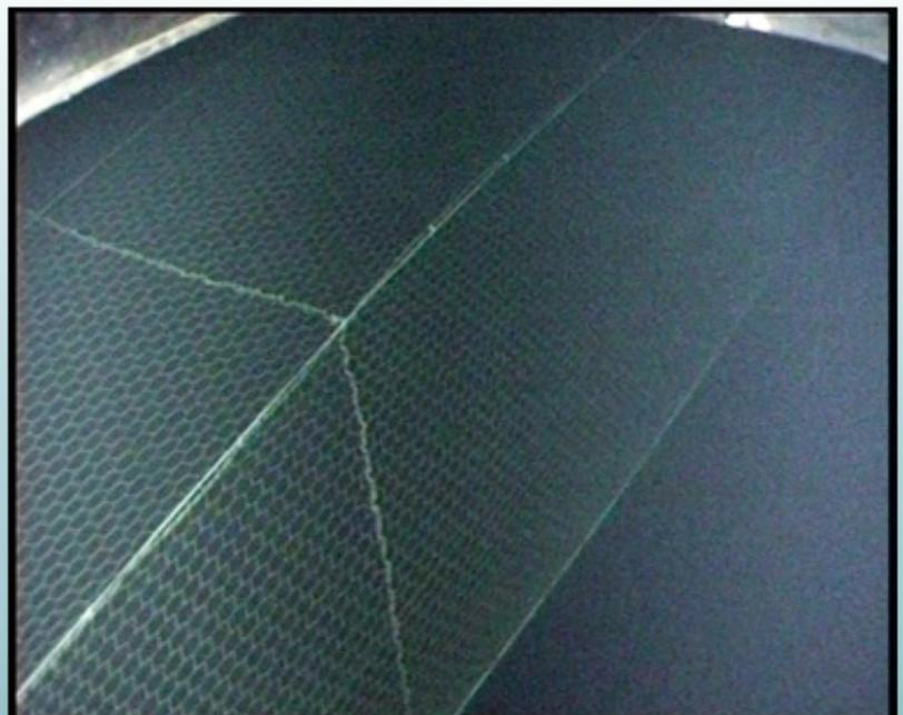
**Figure 5.8:** Aft trawl belly made from brick-shaped meshes.
