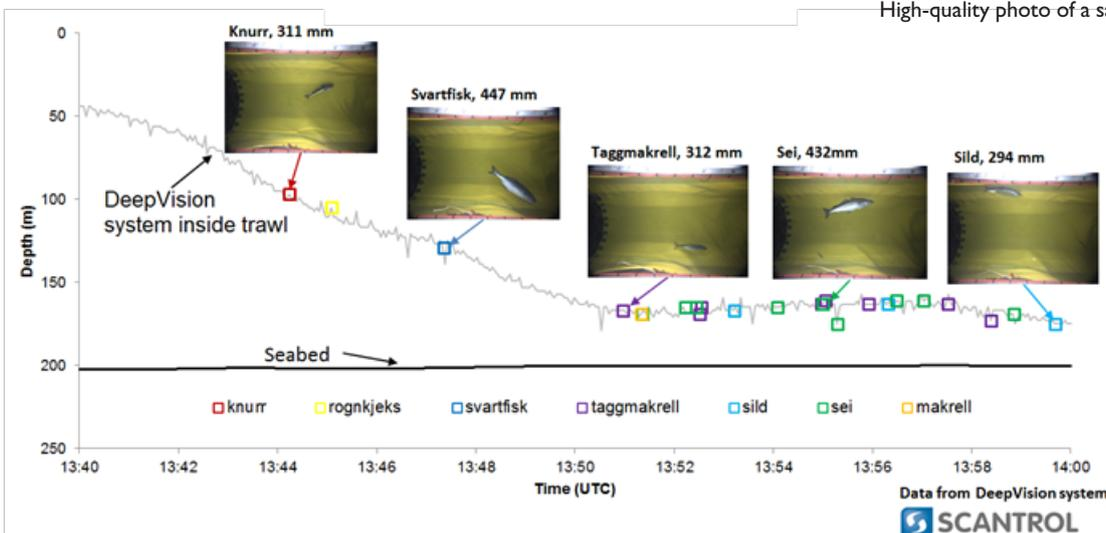
Figure 5.6: Information collected by DeepVision during trawling, showing species and size distribution at various depths.
