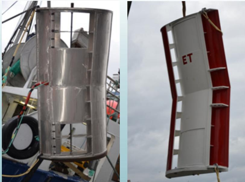
**Figure 5.7:** 2 m<sup>2</sup> (left) and 9 m<sup>2</sup> (right) trawl doors equipped with hatches, which are used to adjust depth and horizontal spread.
