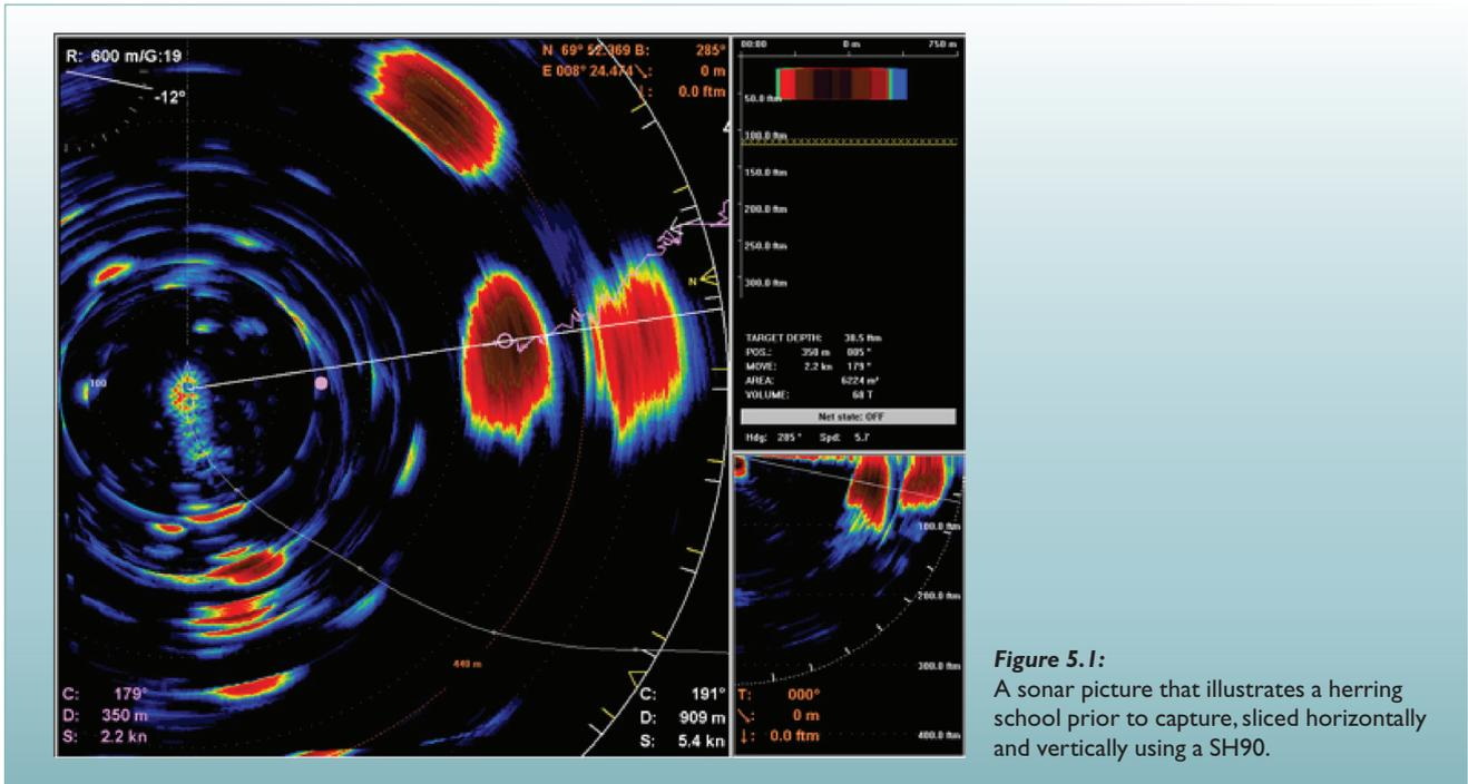
**Figure 5.1:** A sonar picture that illustrates a herring school prior to capture, sliced horizontally and vertically using a SH90.
