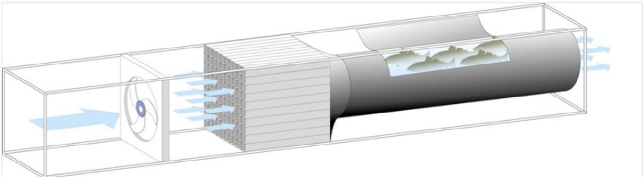
**Figure 5.10:** Sketch of the large swimming tunnel for experimental studies of live fish. The swimming tunnel will be about 6 x 0.9 x 0.9 m and have a total weight in air of about 800–940 kg. It will be placed inside a sea-cage at Tromsø Aquaculture Research Station outside Tromsø, Norway.
