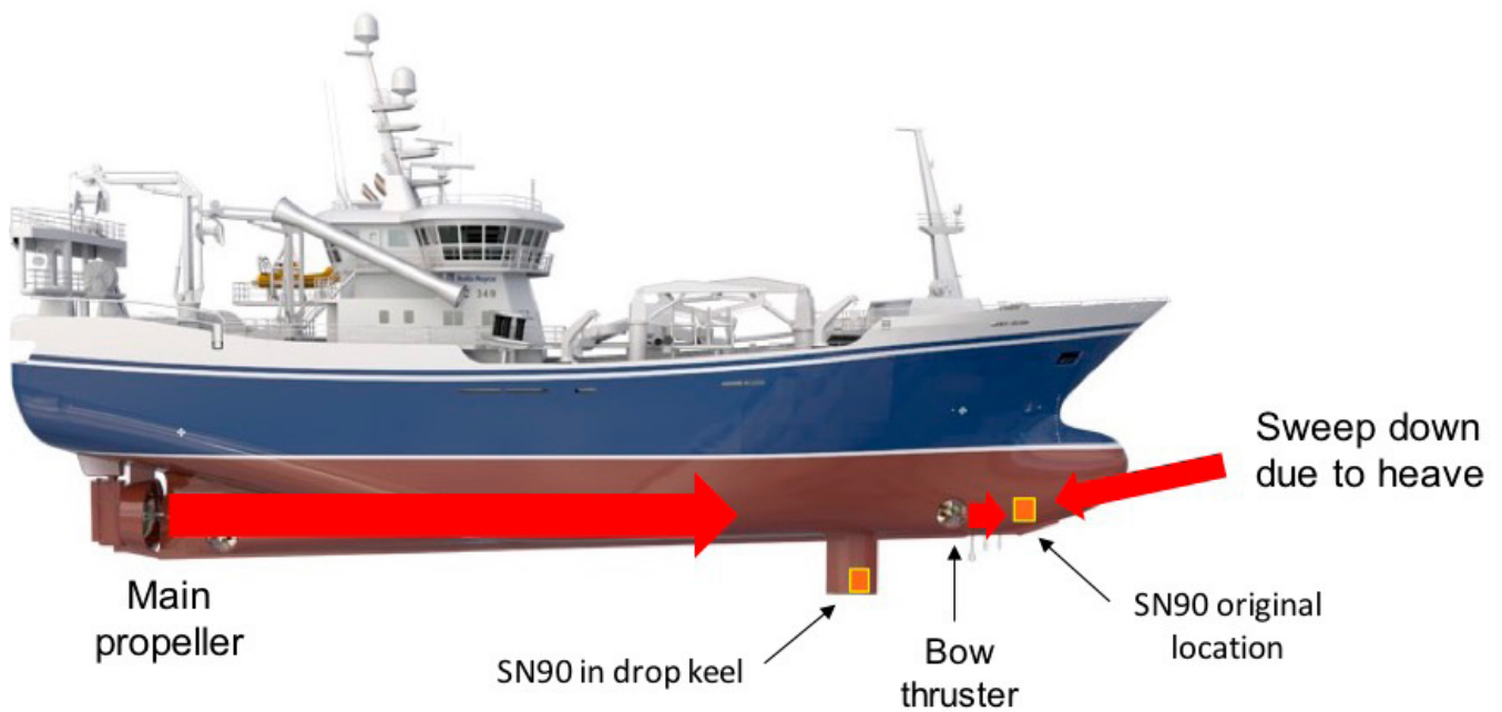
Figure 1. New location of the SN90 transducer in the protruding keel of FV "Eros", 3 m below the vessel hull. The original location closer to the bow attached to the vessel hull is also shown, where it was more exposed to the air bubbles from bow thruster, main propeller and sweep down from vessel heave (picture source: Rolls-Royce, ship design)
