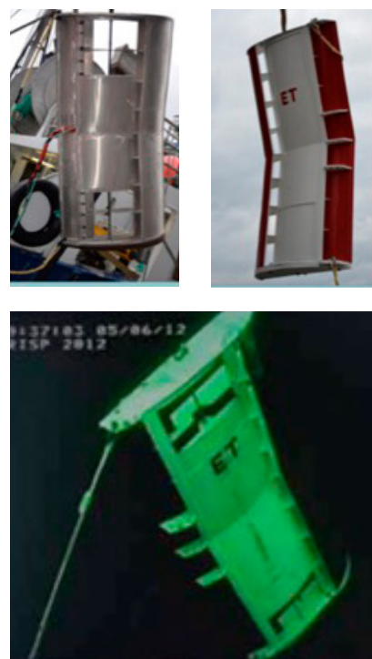
Figure 1. Maneuverable pelagic trawl doors with hatches above and below the towing brackets developed in CRISP. The hatches are opened and shut with an engine controlled over an acoustic communication system.
