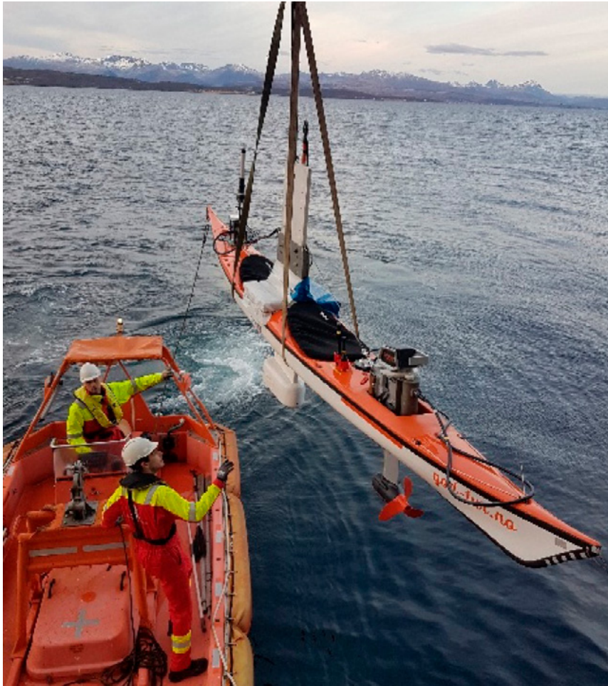
KayakDrone used to measure herring layers in Kværnangen, 2018. The herring reaction to the research vessel was studied and quantified and compared with four other measuring methods.
