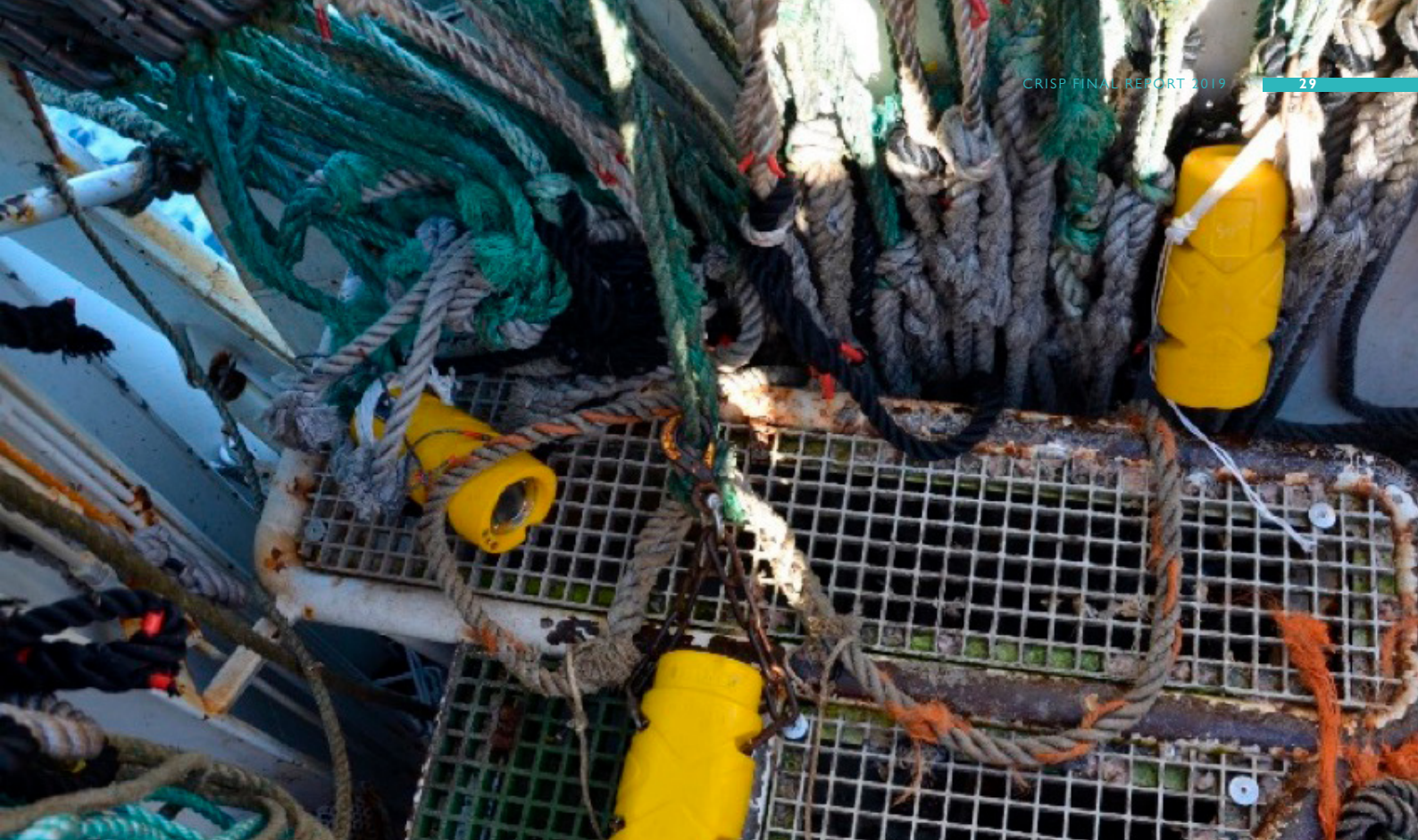
Figure 4. Three positioning transponders attached to the lead-line of a purse seine.
