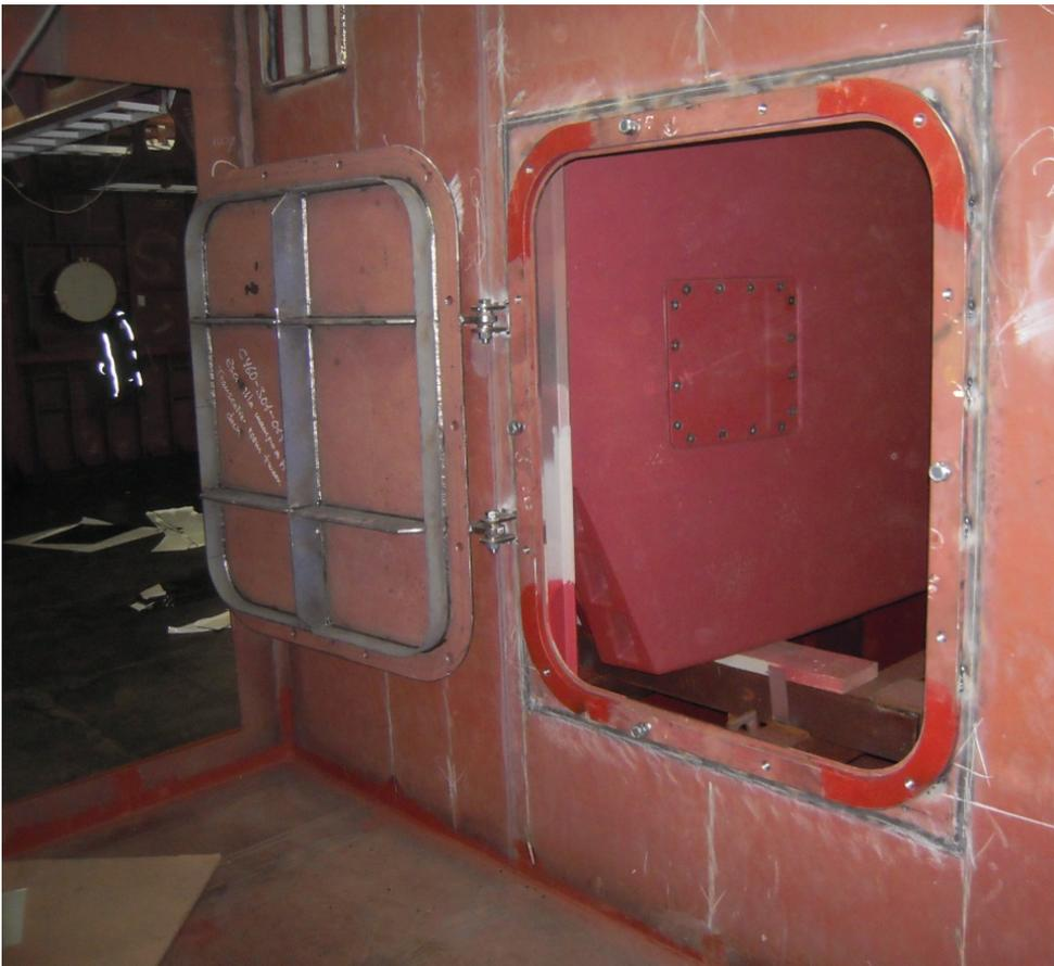
**Trunk with Propeller inspection window and "box" for camera w/light**
