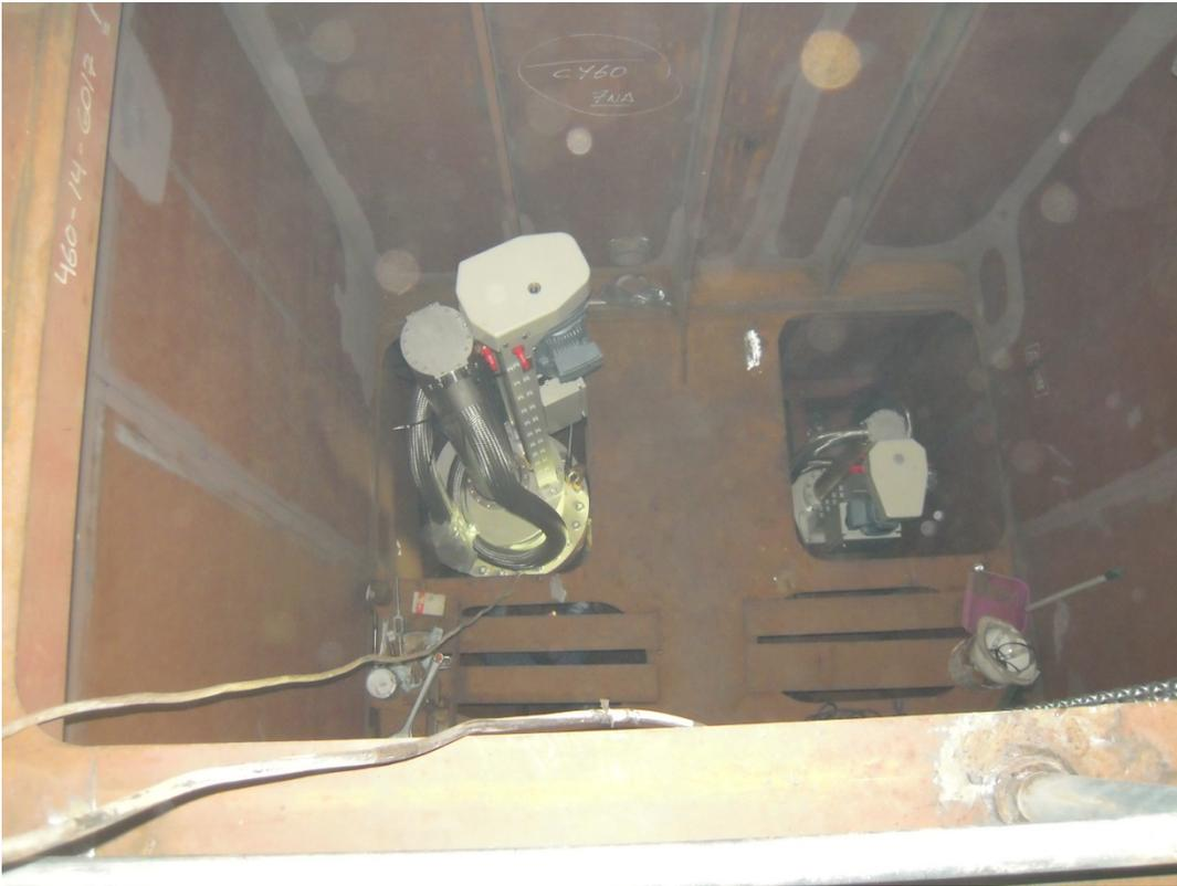
Hatch from Lab 26 to drop keel trunk
