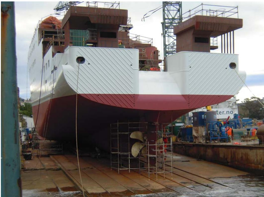
**BL 51-52-53 Wheelhouse and top bridge ready on berth— to be installed after launch**
