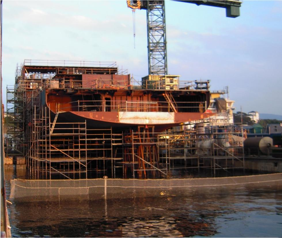
**Bow area has reached full height - Anchors with chain on site.**
