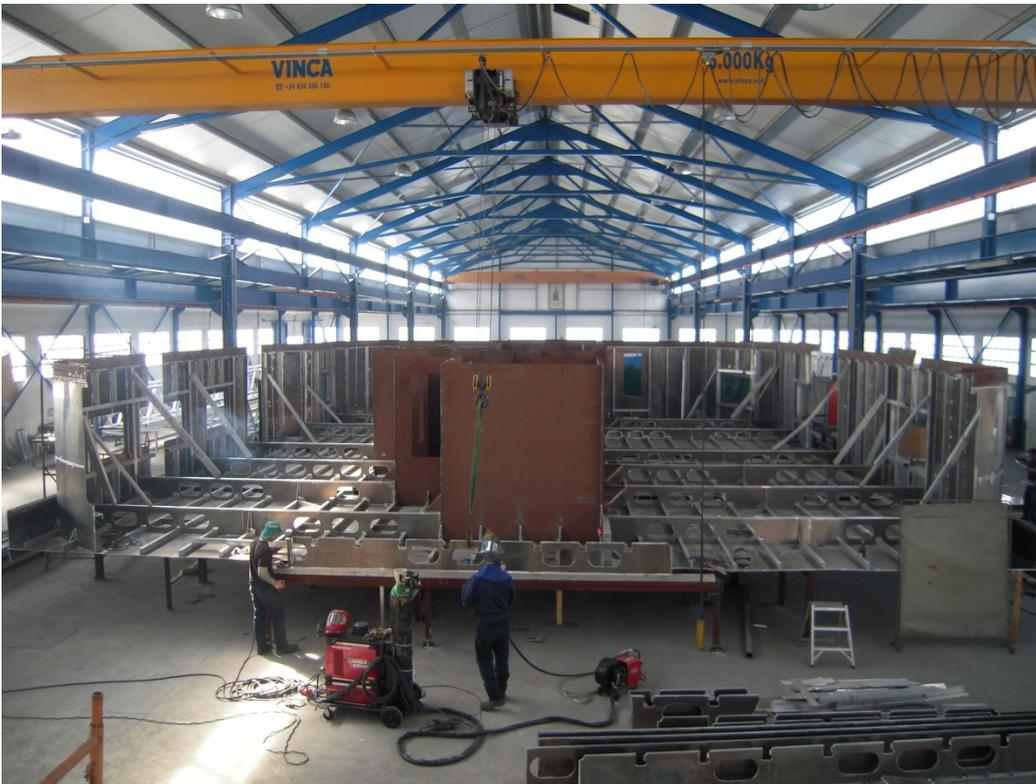
**Steel casing in middle is due to fire regulation**
