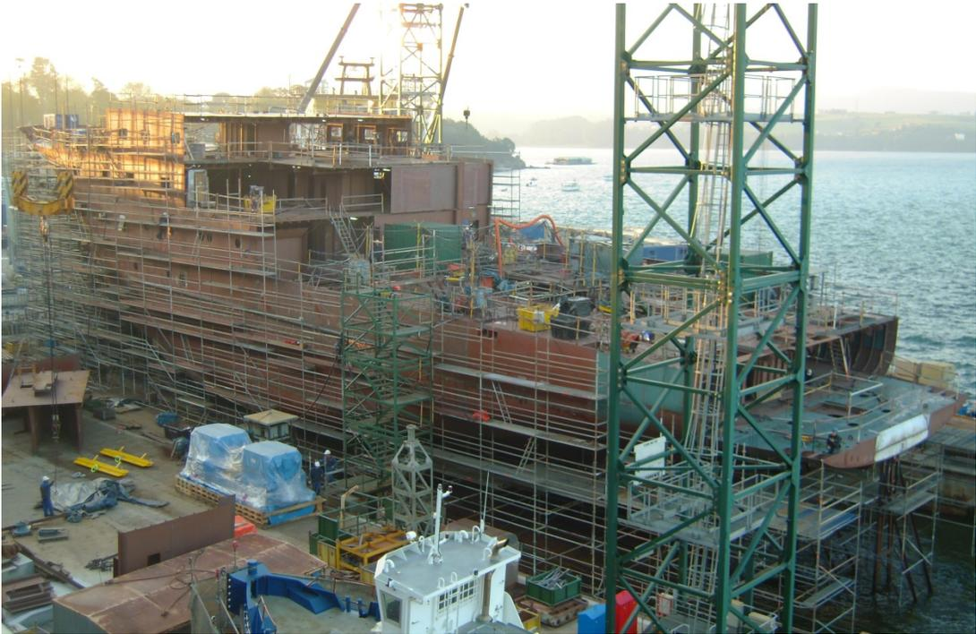
**Slipway 30.09 BL 44 (2<sup>nd</sup> dk) installed – (2 more decks to come on top of this!)**
